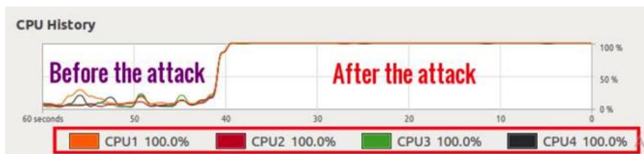
Figure 3.1 CPU Utilization of the client before and after the Cryptojacking Attack. The axes X and Y, respectively, show the running time and percentage of CPU utilization
