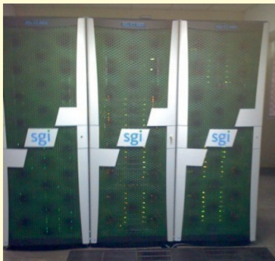
Figure 4.3 Altix ICE cluster system with 96 nodes of Intel Westmere-EP Hex core processors running at 2.93 GHz frequency with 12 MB L3 cache. The 6th largest super computer in the country.
